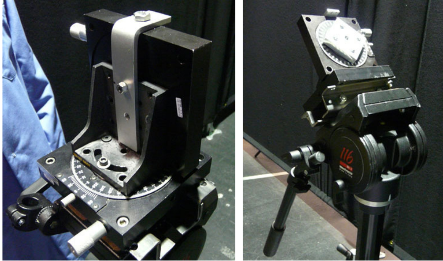
Figure 60: Roll/Yaw Tripod Mount provided by Neptec
