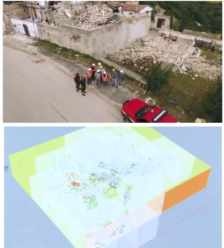
Figure 2.3 [ABOVE] Drones used to assess earthquake damage in Italy (2016) [BELOW] Digital scans are compared to detect movement
