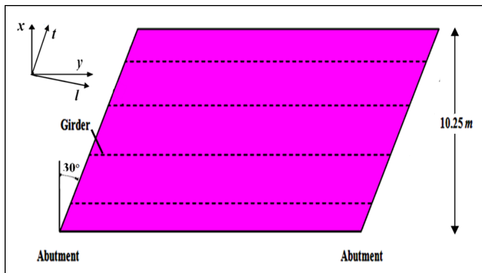
Figure 5.32: Integral bridge without cross bracing (N-1).
