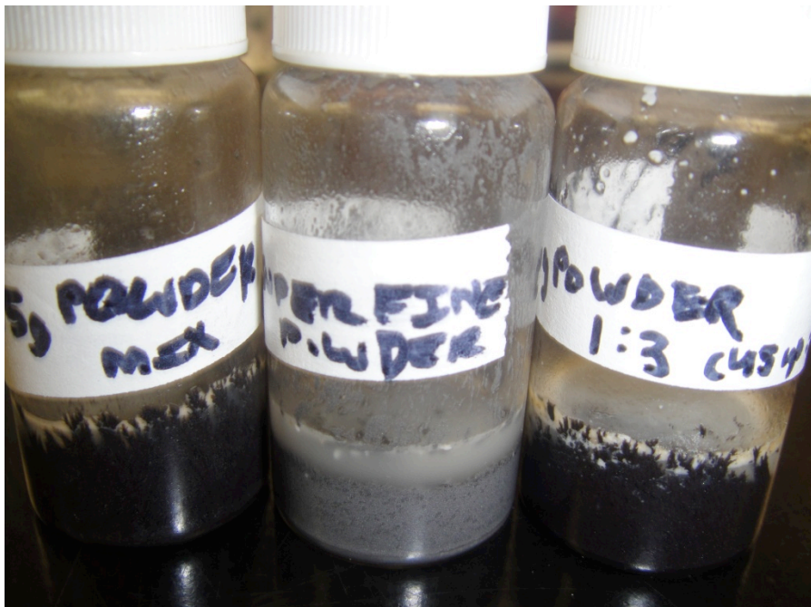
Vial Test with Various Powder Sizes
