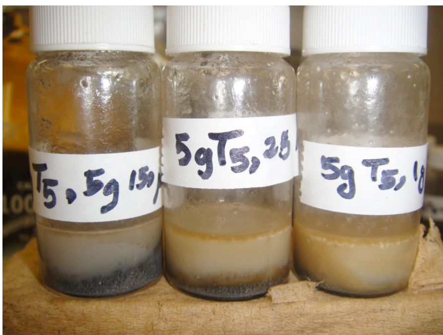
Vial Test Magnetic Powder Dosage Trial
