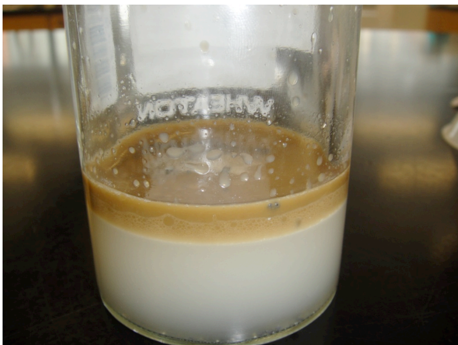
Vial Test (Larger Scale) with Low Magnetic Powder Ratio
