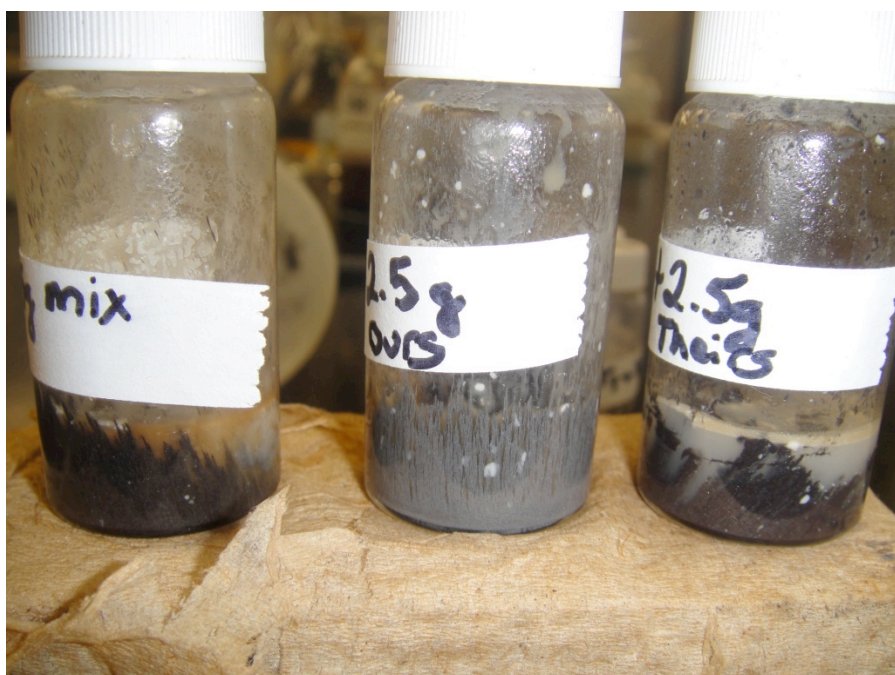
Vial Test with magnetic Field and Artificial Wastewater
