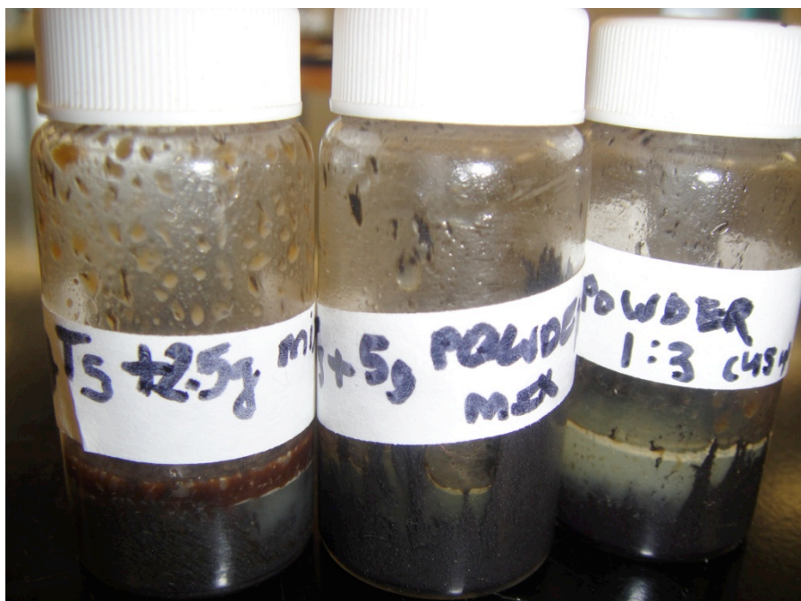
Vial Test Different Magnetic Powder Ratios Trial
