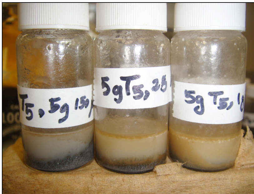
Figure 4.4 Vials holding artificial wastewater and various magnetic powder sizes
