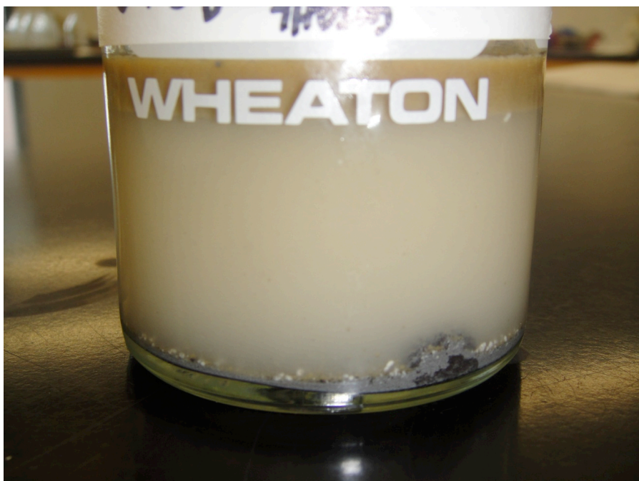
Oil/Powder Flocs in Vial Test (Larger Scale)
