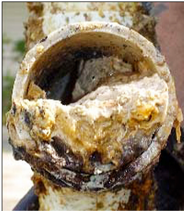
Figure 2.2 “Oily wastewater build-up” in pipelines
