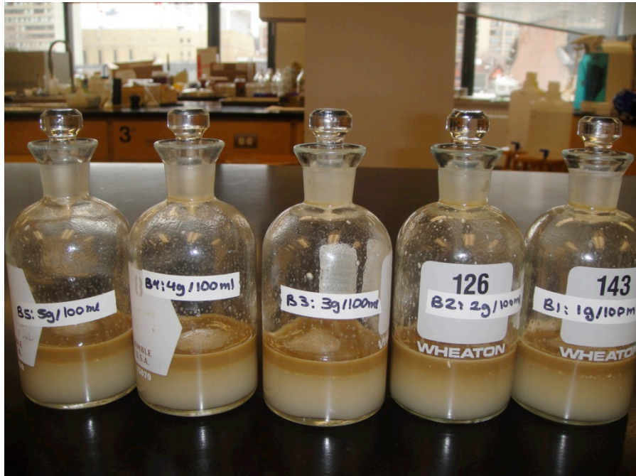
Vial Test (Larger Scale) with Various Powder Ratios
