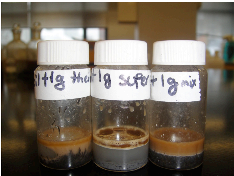
Vial Test with Different Grades of Magnetic Powder
