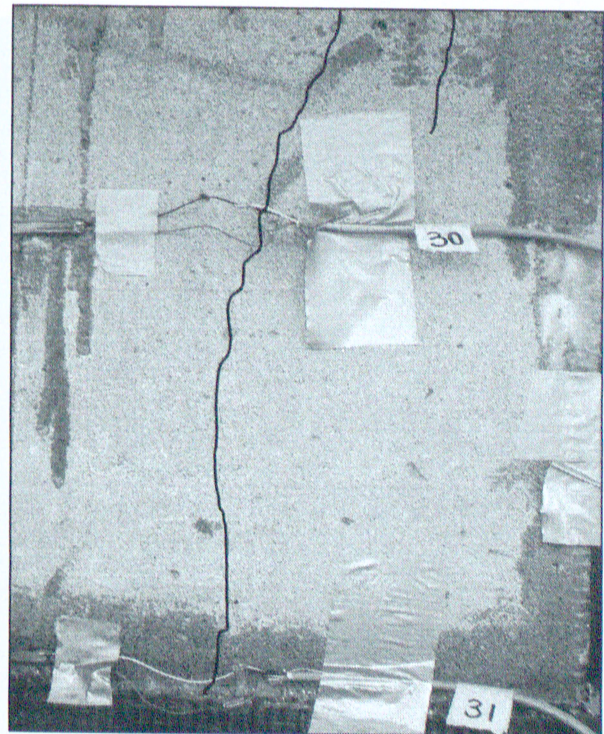
Figure 3.80 – Cracks at midspan portion on south (left) and north (right) faces
