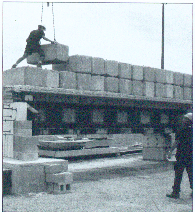
Figure 3.68 – Second row of loading (left), and positioning (right)
