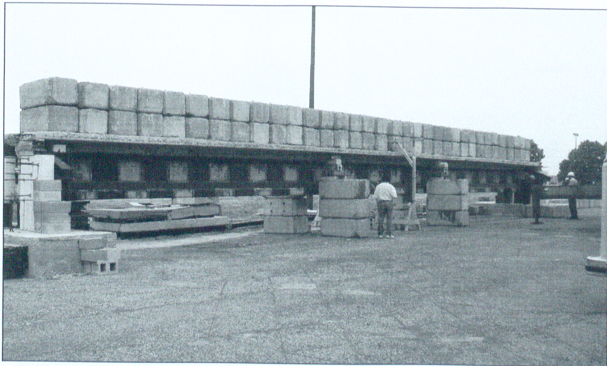
Figure 3.70 – Completion of first two rows of one ton block loading
