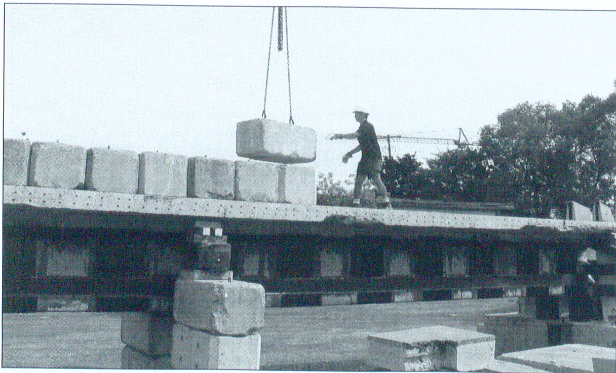
Figure 3.66 – First row of loading: one ton blocks
