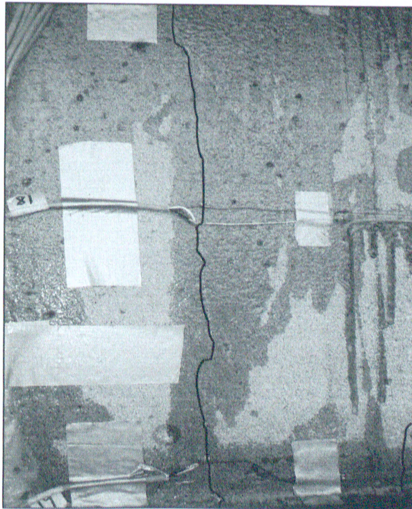
Figure 3.80 – Cracks at midspan portion on south (left) and north (right) faces
