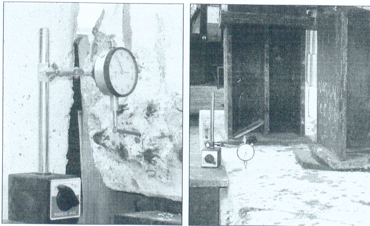
Figure 3.59 – Mechanical dial gages, at supports, for bearing pad (left) and foundation (right) settlement
