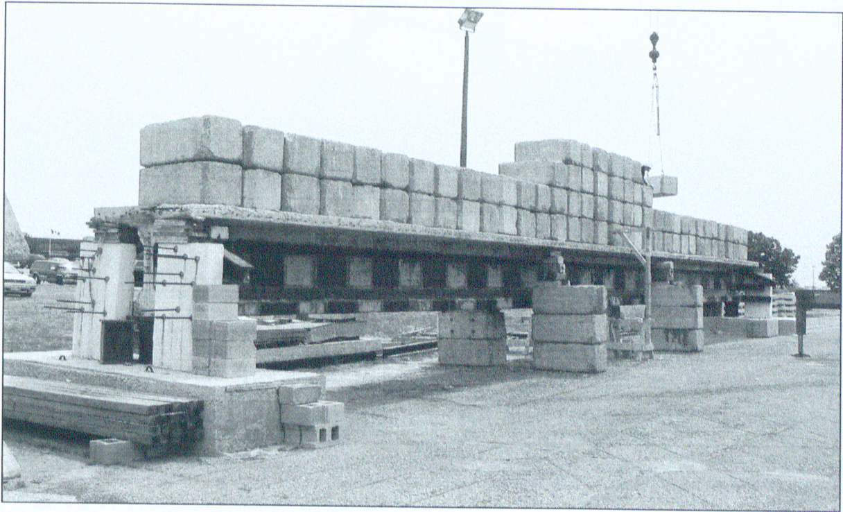
Figure 3.71 – Third and fourth rows of loading: one ton blocks
