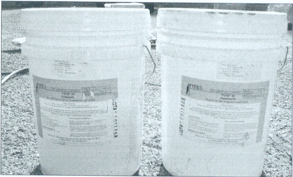
Figure 3.32 – Component A and B resin mix for Tyfo® TC - Tack Coat Epoxy
