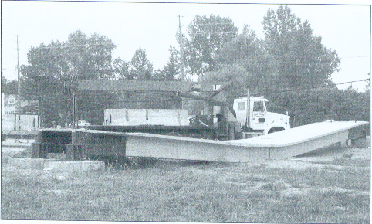
Figure 2.15 – DT-100 girder after ultimate failure loading (Cofini, 2005)
