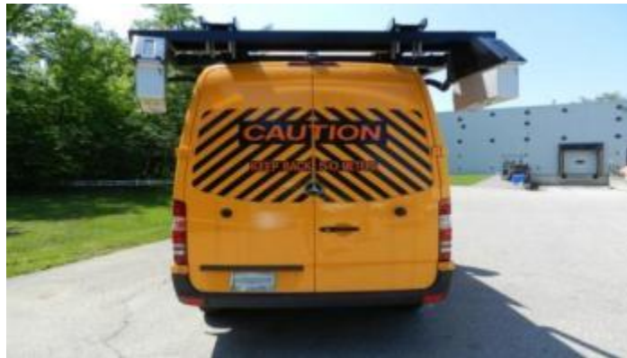
Figure 2. Laser rut measurement system (MTO 2016)
