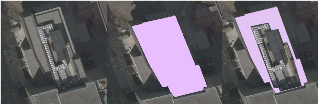
Figure 2. CED building –orthophoto, digitized gross area and usable area
