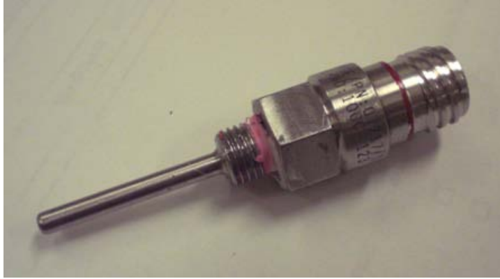
Fig. 5.6 RTD temperature sensor, supplied by Honeywell
