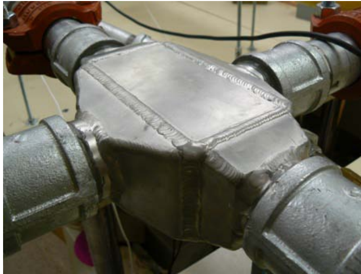
Fig. 5.3 Air to air plate-fin heat exchanger, manufactured by Bell Intercoolers
