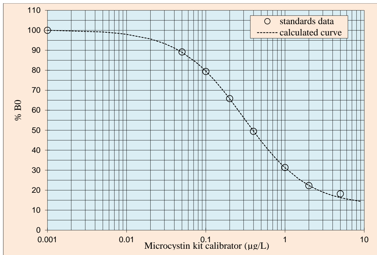
FIG G1. STANDARD CURVE FOR THE CALCULATION OF MICROCYSTINS
