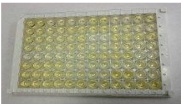
FIGURE 23. MICROTITER PLATE WITH 96-WELLS FOR ELISA
