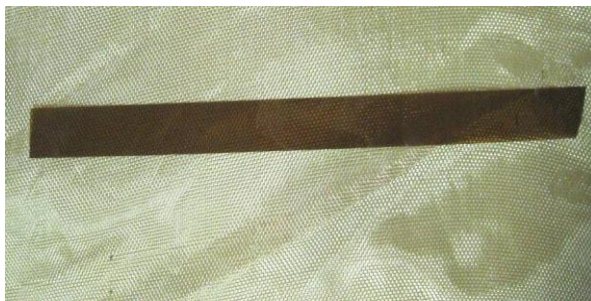
Figure 4.10 Upilex Tensile Test Specimen
