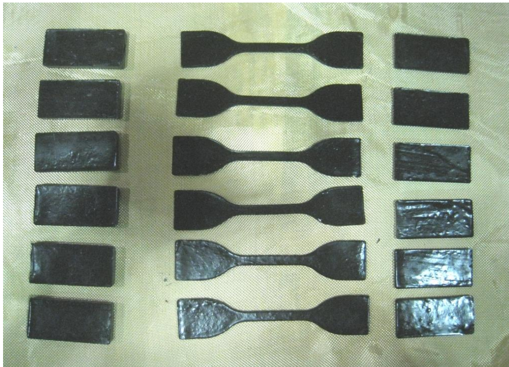
Figure 4.12 PR 1422 Class B Hardness, Tensile, and Volume Swell Specimens
