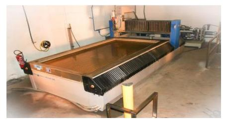
Figure 4-18: Water jet cutting machine (source: Antech Technologies Inc.)
