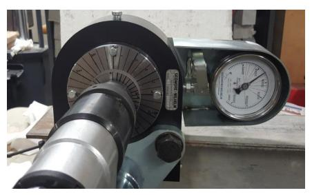
Figure 4-22: Wilhelm Skidmore bolt tensioning device prepared for clamping force verification test
