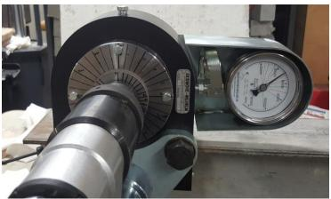
Figure 4-23: Wilhelm Skidmore bolt tensioning device prepared for clamping force verification test at 120° of a turn.
