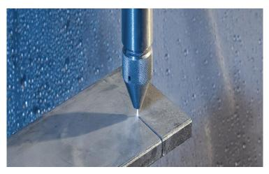
Figure 4-19: Water jet-cutting process (source: Ant Applied New Technologies – AG)
