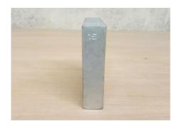
Figure 4-21: Galvanized plate with label number stamped in the side before hot dip galvanization process
