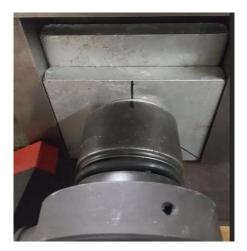
Figure 4-34: Alignment of the electric torque wrench with zero mark on front plate of specimen
