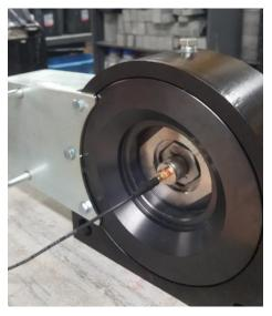
Figure 4-5: Attachment on the Mini-Max ultrasonic bolt elongation measuring device to torqued bolt head inside of Skidmore Wilhelm machine
