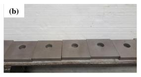
Figure 4-26: Specimen plates arranged to be final surface treated (a) galvanized plates to be wire brushed and (b) blasted clean surface to be cleaned with a regular brush to remove
