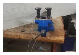
Figure 4-12: Attachment of Type K-thermocouple wires to the head of bolts
