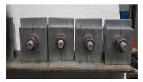
Figure 4-31: Rotation of centre plate of specimen assembly hot-dip galvanized plates with galvanized bolts
