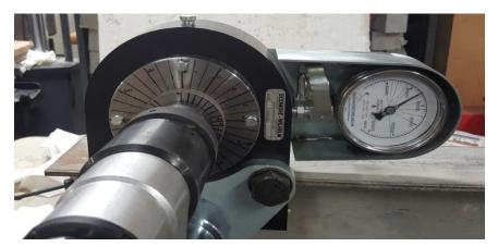
Figure 4-4: Incremental torqueing of structural bolt using Skidmore Wilhelm machine and electric torque wrench
