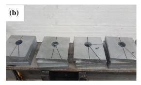
Figure 4-28: (a) Galvanized plates with galvanized bolts been scribe with 160<sup>0</sup> stencil and (b) Galvanized plates with A325 bolts been scribe with 152<sup>0</sup> stencil.
