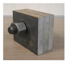
Figure 4-29: Typical initial assembly of three plate of a specimen with 7/8" diameter bolt
