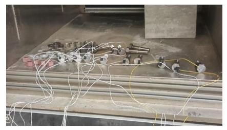
Figure 4-14: View of bolts, washers and nuts placed inside environmental chamber
