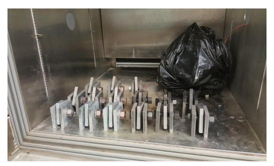
Figure 4-39: Placement of dry-fitted sample inside of environmental chamber
