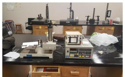
Figure 4-20: Equipment and method use for the determination of surface roughness
