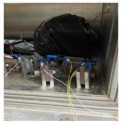
Figure 4-40: Placement of insulating foam to back of K-thermocouple wire, then replacement of specimen into environmental chamber
