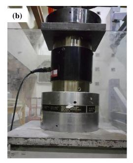
Figure 4-35: (a) MTS Hydraulic Universal Testing machine and (b) 500 kN capacity portable load cell
