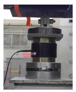
Figure 4-36: Compressive loading of centre plate of specimen assembly during slip testing
