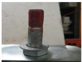
Figure 4-7: Application of multi-purpose grease lubricant to the threads of galvanized bolt
