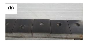
Figure 4-27: Specimen plates arranged to be final surface treated (a) A1010 clean mill scale surface to be cleaned with acetone and (b) 350W Steel clean mill scale to be cleaned with acetone
