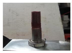
Figure 4-8: Application of multi-purpose grease lubricant to the threads of stainless steel
