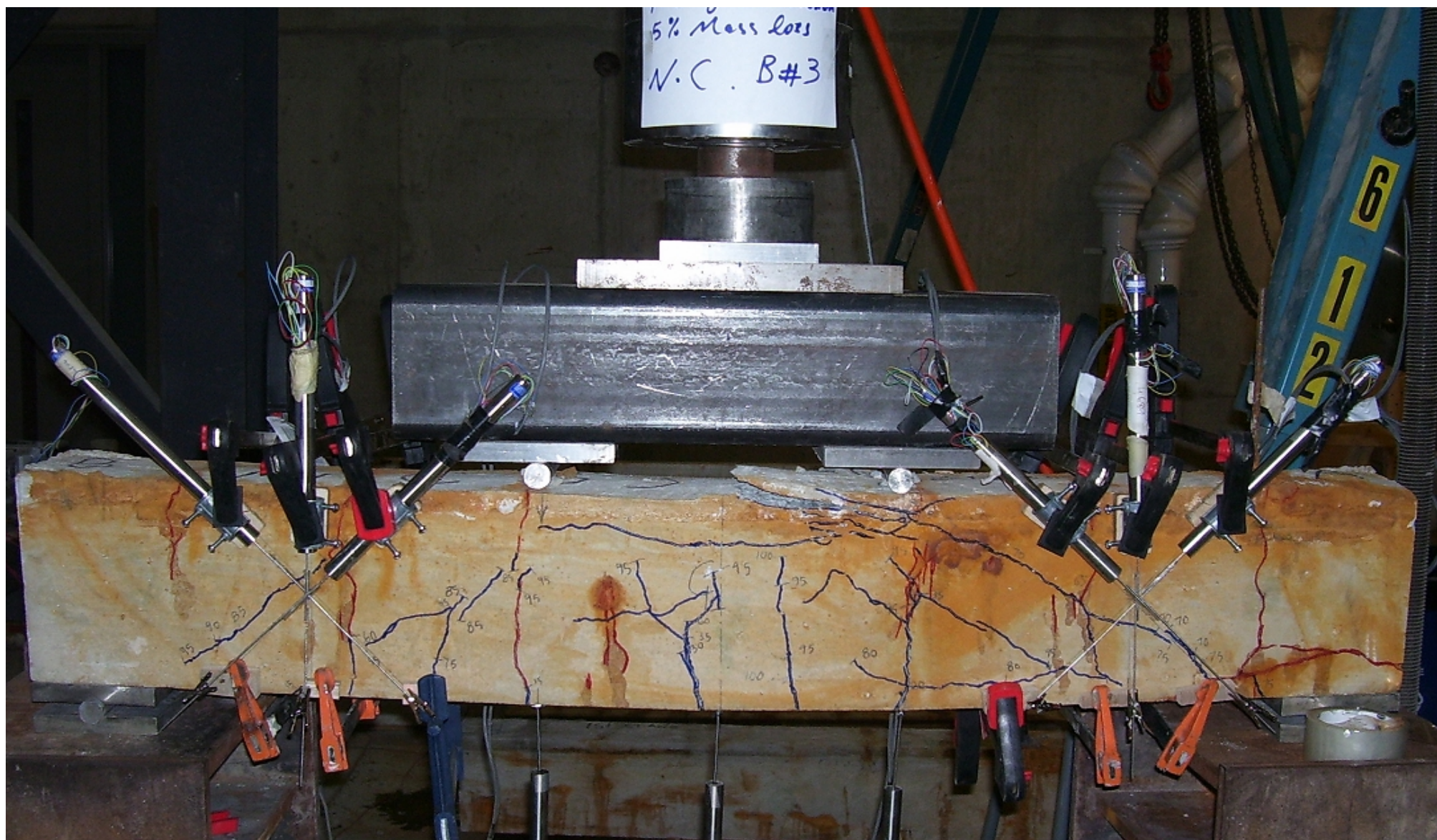
Figure (C-5): Loading cracks pattern for NC beam no.3 with 5% mass loss.
