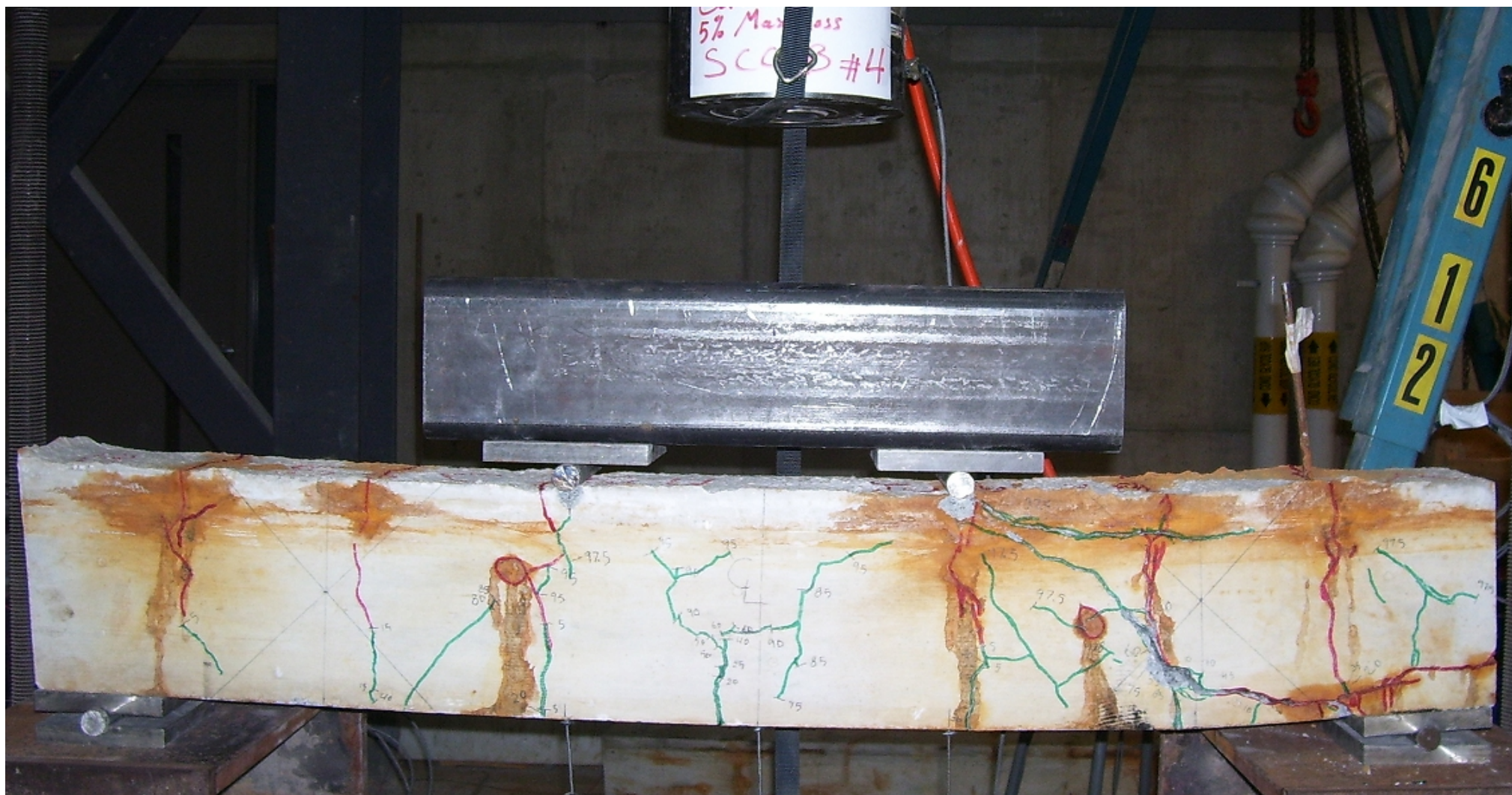
Figure (C-7): Loading cracks pattern for SCC beam no.4 with 5% mass loss.
