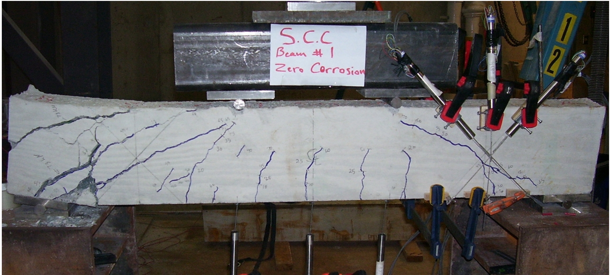
Figure (C-3): Loading cracks pattern for SCC beam no.1 with zero mass loss.
