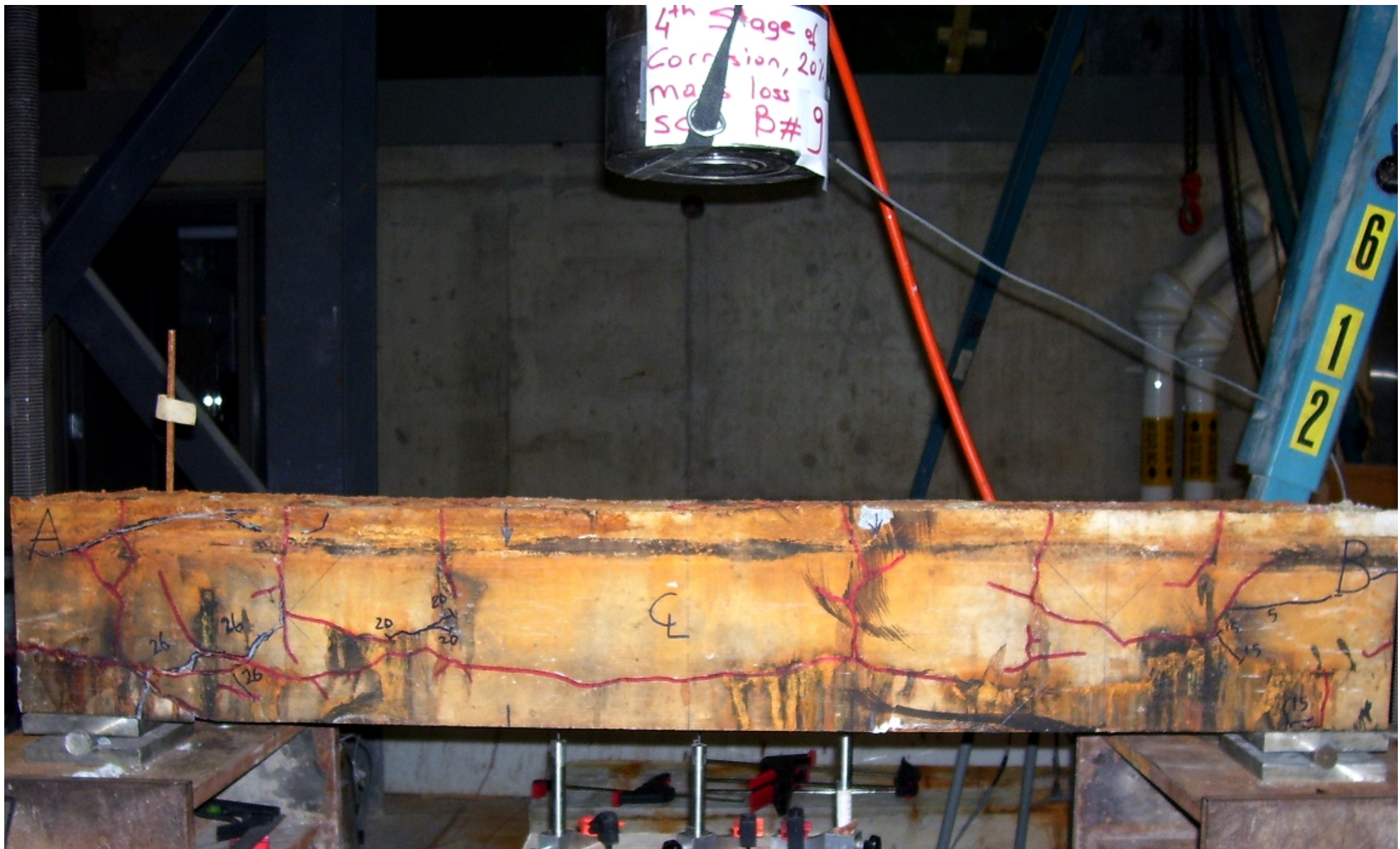
Figure (C-20): Loading cracks pattern for SCC beam no.7 with 20% mass loss.
