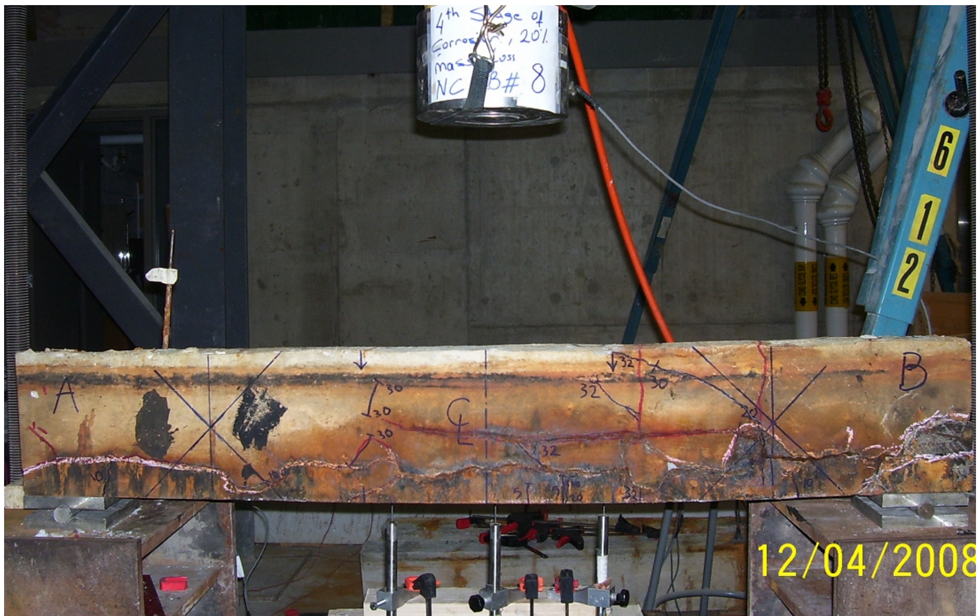
Figure (C-18): Loading cracks pattern for NC beam no.8, with 20% mass loss.
