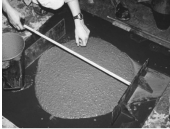
Figure (2-29): SCC slump flow (ACI 237R-07).
