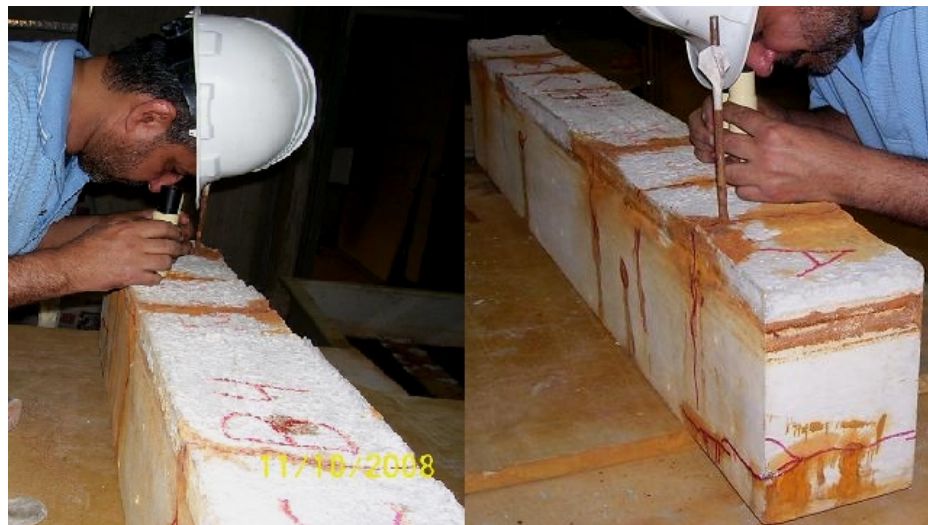
Figure (3-8): Measuring the crack widths on the corrosion cracks pattern.
