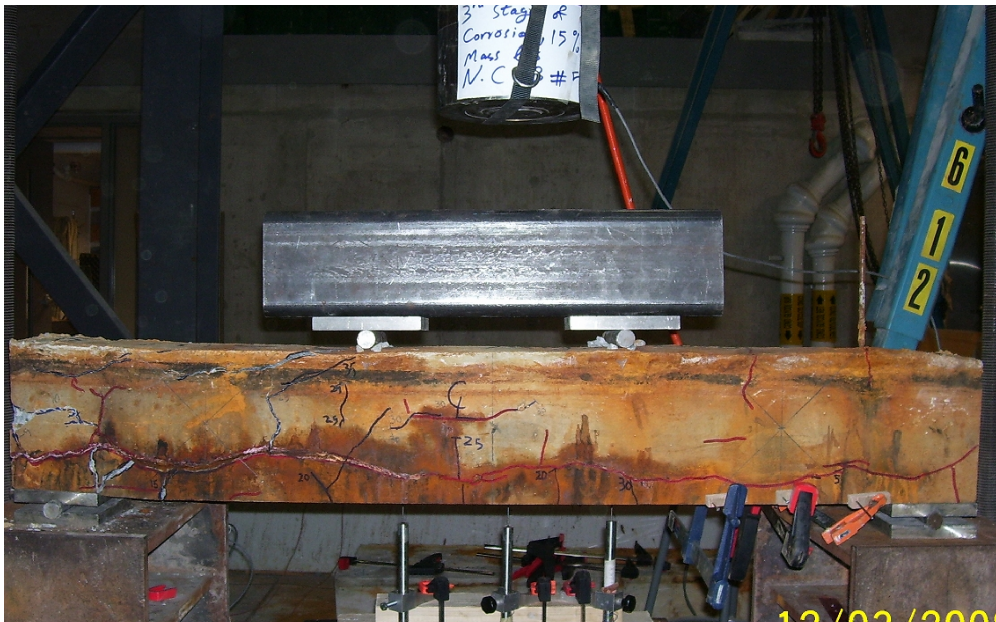
Figure (C-14): Loading cracks pattern for NC beam no.5 with 15% mass loss.
