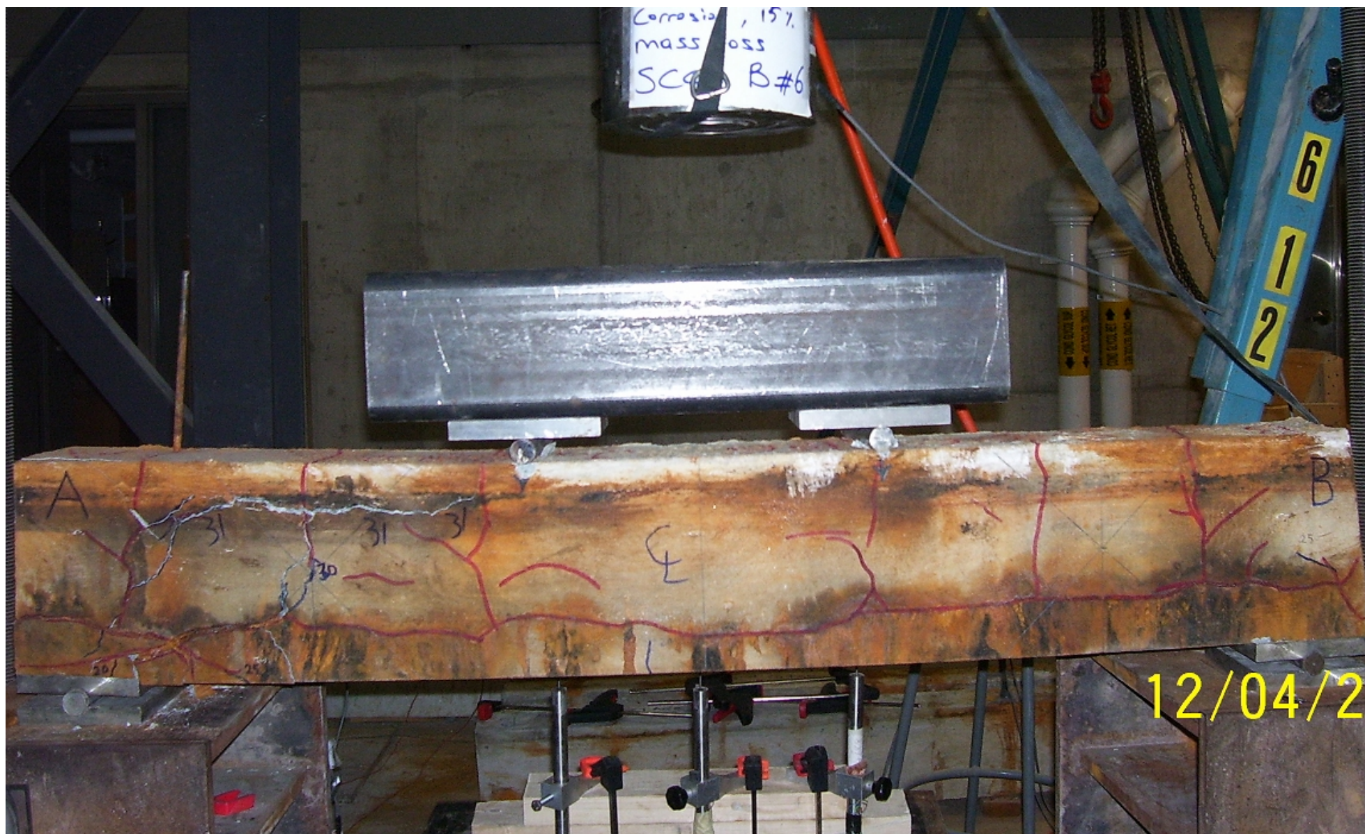
Figure (C-15): Loading cracks pattern for SCC beam no.6 with 15% mass loss.
