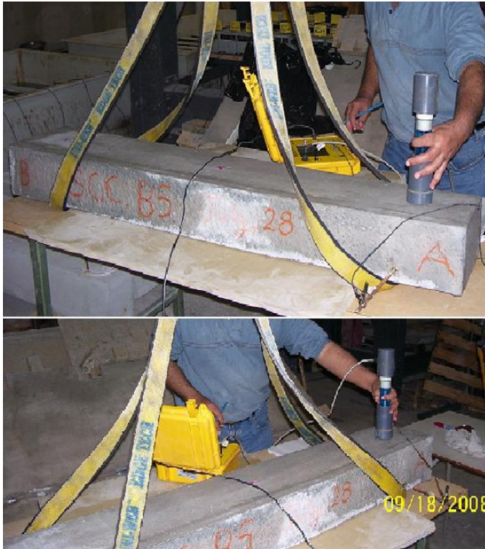
Figure (4-1): Half-cell potential test applied on NC and SCC beams numbered 3 - 10.
