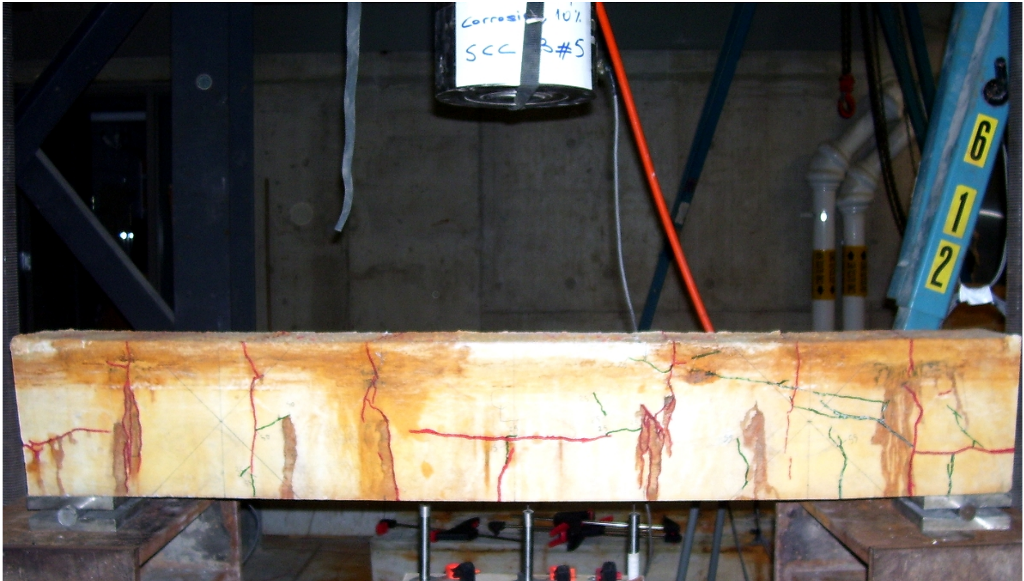
Figure (C-11): Loading cracks pattern for SCC beam no.5 with 10% mass loss.
