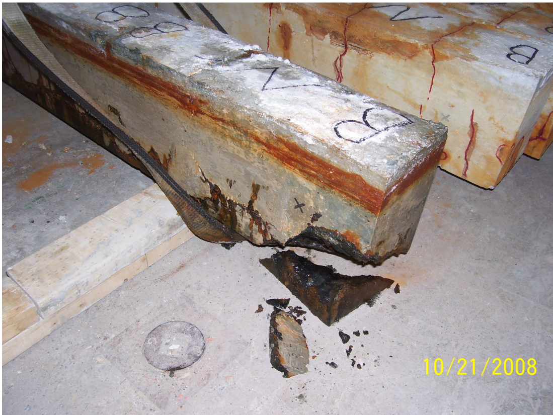
Figure (3-9): Spalling of concrete from the bottom of specimen NC B-8.
