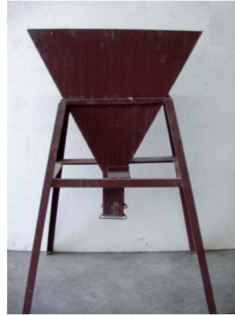
Figure (2-32): Schematic of V-funnel apparatus (Khayat, 2004). Photo on right (Abdul Hameed, 2005).
