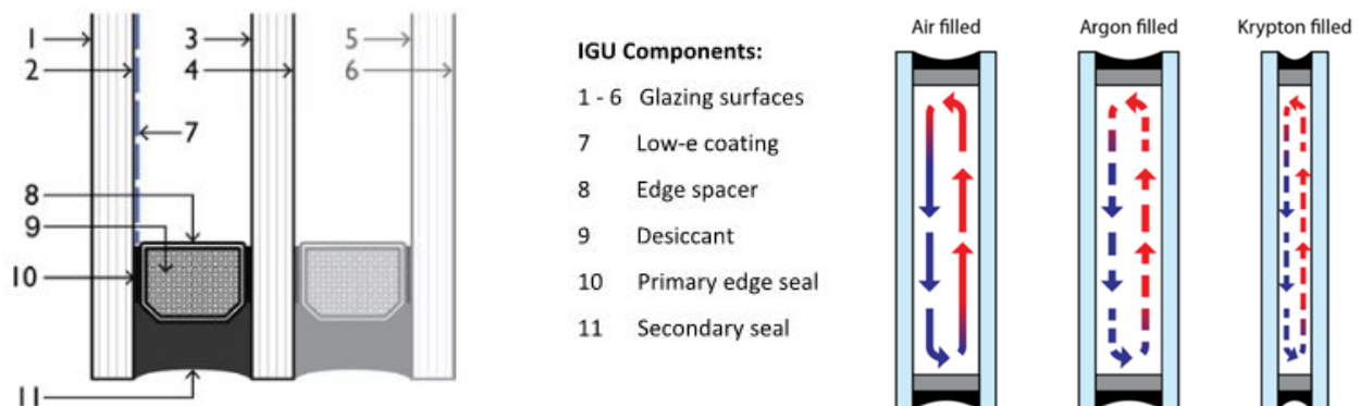
Figure 2.8: Typical components of IGU and Low conductance gas fills (RDH, 2017)
