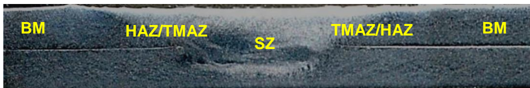
Figure 2.2: Cross section of a FSLWed AZ31B-H24 Mg alloy indicating the ‘welding zones’ of FSW [74, 78, 79].
