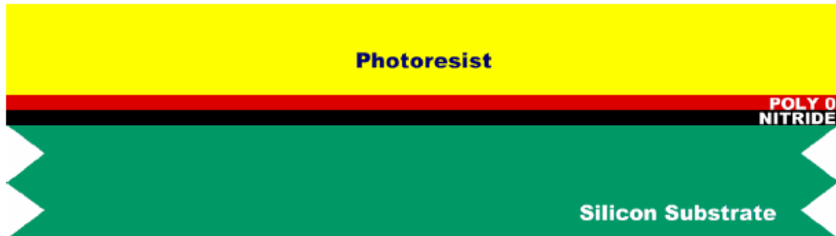
Figure 6. Nitride, Poly0 and Photoresist layers deposited on the Silicon wafer substrate [11]
