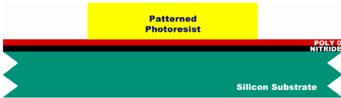
Figure 7. The Photoresist Layer patterned using Photolithography [11]
