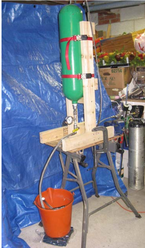
Figure 7.1: Injector flow test setup
