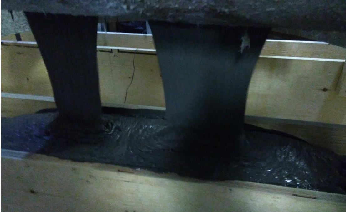
Figure 21: High flowability of UHPFRC
