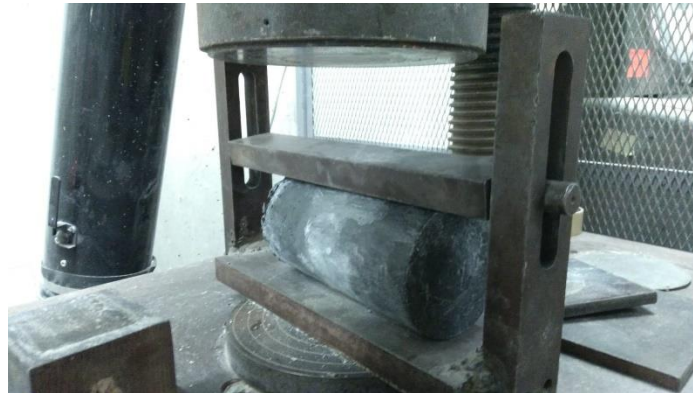
Figure 24: Splitting tensile test preparation
