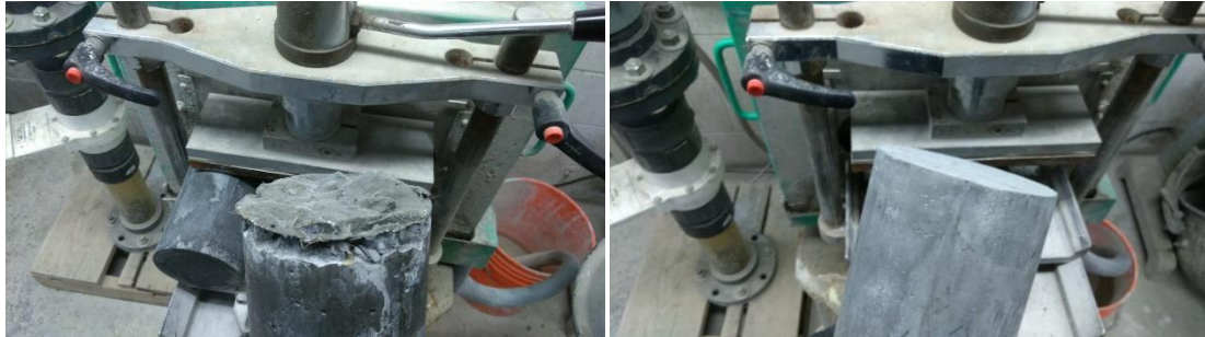
Figure 22: Cylinder end grinding; before (left) and after (right)
