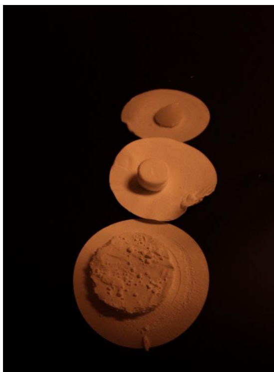
Figure 6.2 Final products attained after hydrothermal synthesis using different co-solvents;. 80EG-150-3 (larger cylinder, front facing); 80DEG-150-3 (compact cylinder, middle); 80TEG-150-3 (pellet, back).
