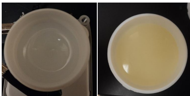
Figure 6.1 Precursor solution using TEG; Initial colour precursor solution: milky white (left side); Final colour precursor solution after 16 hours aging (right side).
