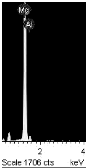
Figure B.1.1. SEM micrograph of AZ91E alloy at the 0.3 wt.% Ti addition level showing a) general microstructure and EDX scans of b) primary \alpha -Mg, c) Mg_{17}Al_{12} , and d) Mn_x-Al_y phases.
