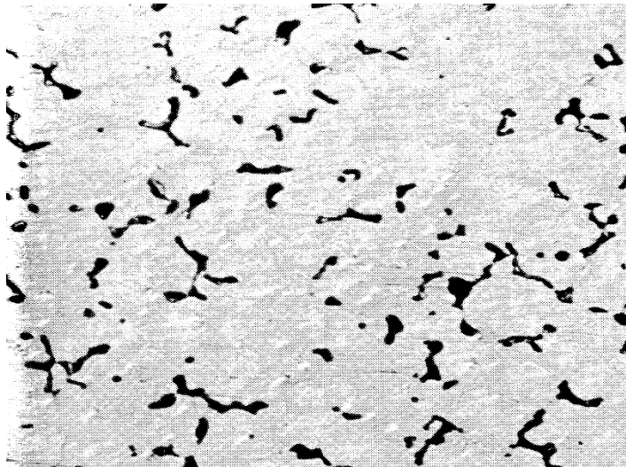
Figure 4. Shrinkage porosity in AZ92 sand casting at 150X magnification [16].
