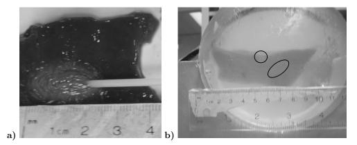
Figure 2. (a) A thermal lesion in bovine liver produced with 805nm laser, (b) liver embedded in gelatin during imaging (position of the lesions are marked)
