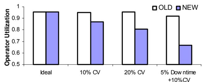
**Figure 2:** Sensitivity of NEW line and OLD dock systems' operator utilization rates to variability in operators' cycle time (10% & 20% coefficient of variation) and to machine downtime (5% downtime) based on flow simulation models.
