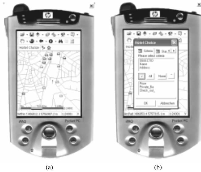
Figure 1. ArcPad desktop emulation showing the filtering and marking of nearby hotels (a) and the selection of criteria by the user (b)
