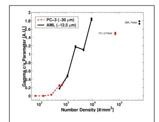
Figure 7. The GG c/v parameter with 95 % confidence intervals for HFUS data from suspensions of AML and PC-3 cells. The number density was determined based on the concentration used and assuming uniform cell sizes. The GG c/v parameter increases with number density for both cell types. This agrees with the interpretation of GG c/v as the effective scatterer number density.
