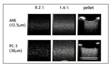
Figure 3. B-scan images (8 x 8mm) of the suspensions of various concentrations of AML cells (top row) and PC-3 cells (bottom row). At the lower concentrations individual cells are apparent, however as the concentration is increased the B-scan shows the speckle pattern characteristic of US images. While the AML pellet appears darker than the 1.6 % concentration solution, the PC-3 pellet does not, implying differences in the scattering interaction in solution vs. pellet.
