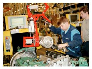
Figure 3: Line operator installing turbo unit sub-assembly using lift assist device.
