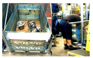
Figure 4: Heavy parts stored in large crates lead to high low back loading and elevated risk for operators.
