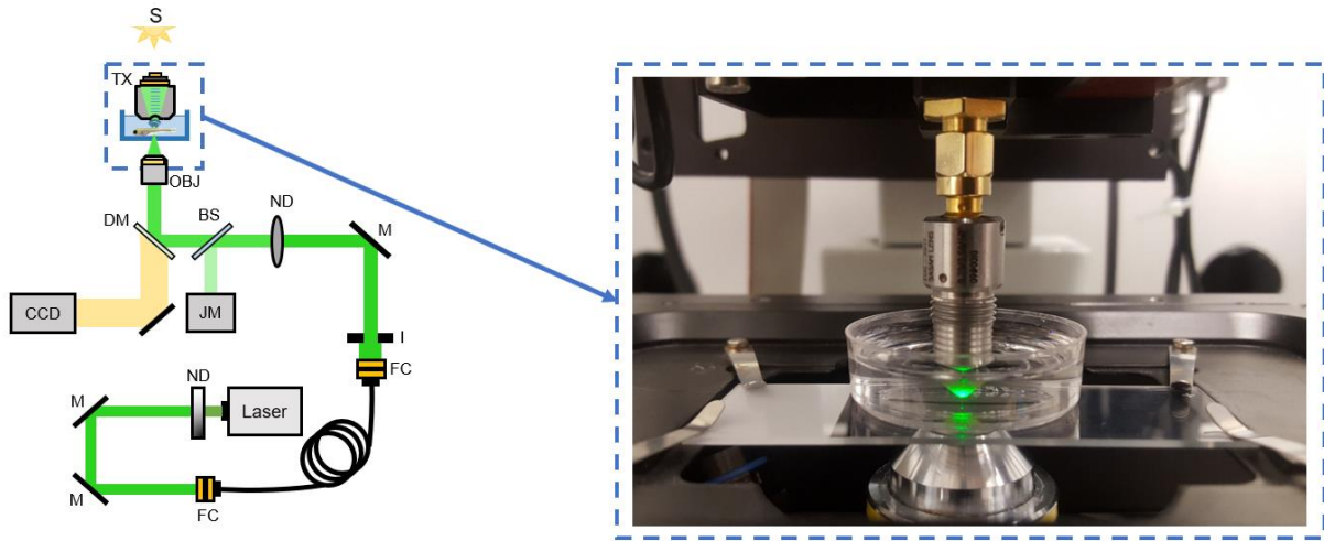
Figure 5.1: Schematic of the experimental setup. A photograph of the components in the dashed box on the left is shown on the right hand side of the image. Abbreviations: ND, neutral density filter; M, mirror; FC, fiber coupler; I, iris; BS, beamsplitter; JM, joulemeter; DM, dichroic mirror; OBJ, objective; TX, transducer; S, brightfield light source.
